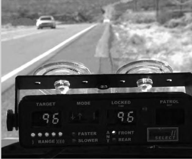
☛)) In very light traffic there's generally little doubt about which target the radar is monitoring. This driver didn't spot the marked cruiser until his speed had been monitored for several seconds.
