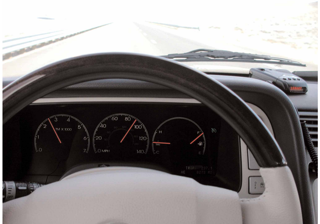
Rule #1 of detector placement: Put it where you can see and reach it and as low as possible.
